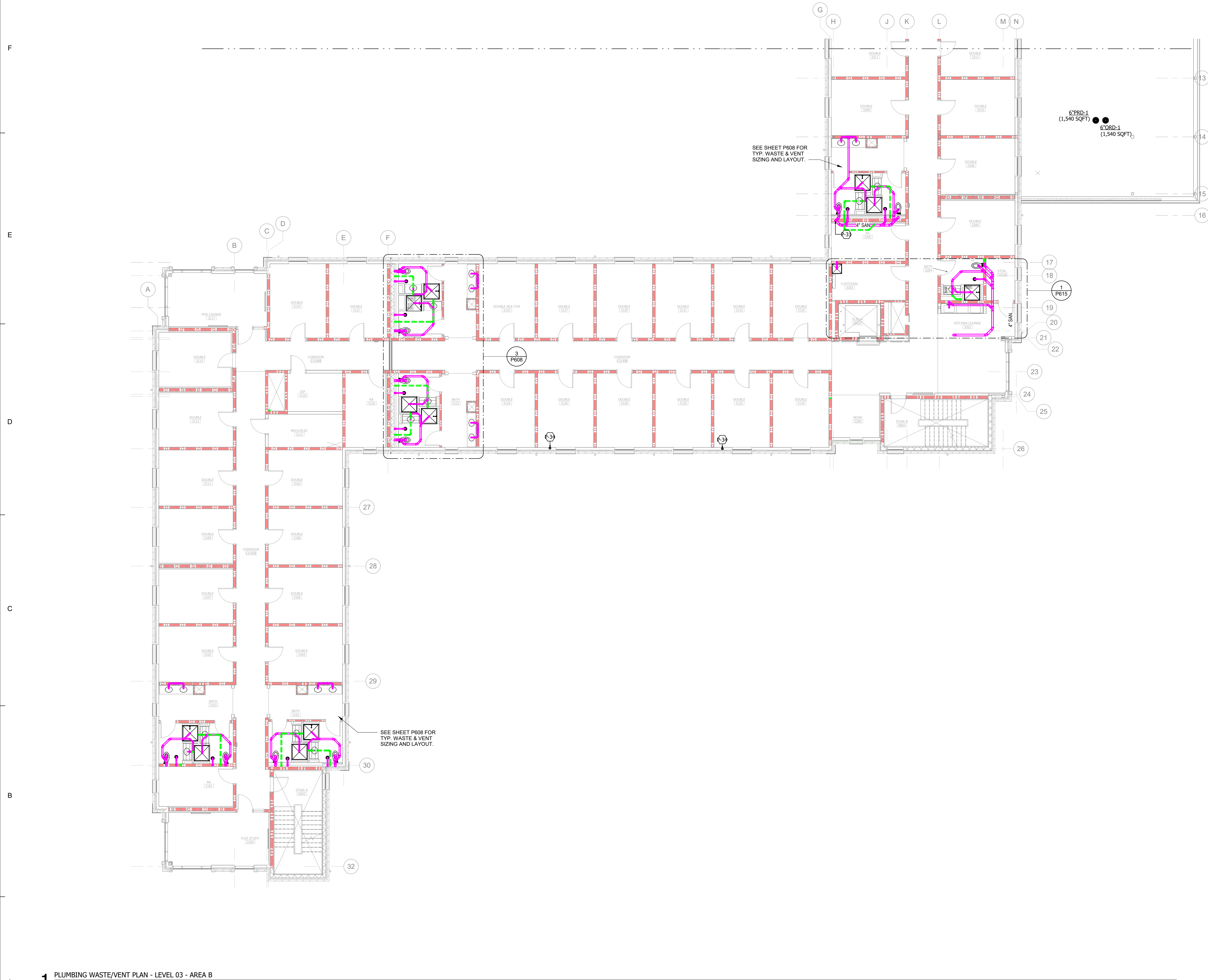
1 PLUMBING WASTE/VENT PLAN - LEVEL 03 - AREA B 0 1' 2' 4' 8' 16' 32' 1/8" = 1'-0"
