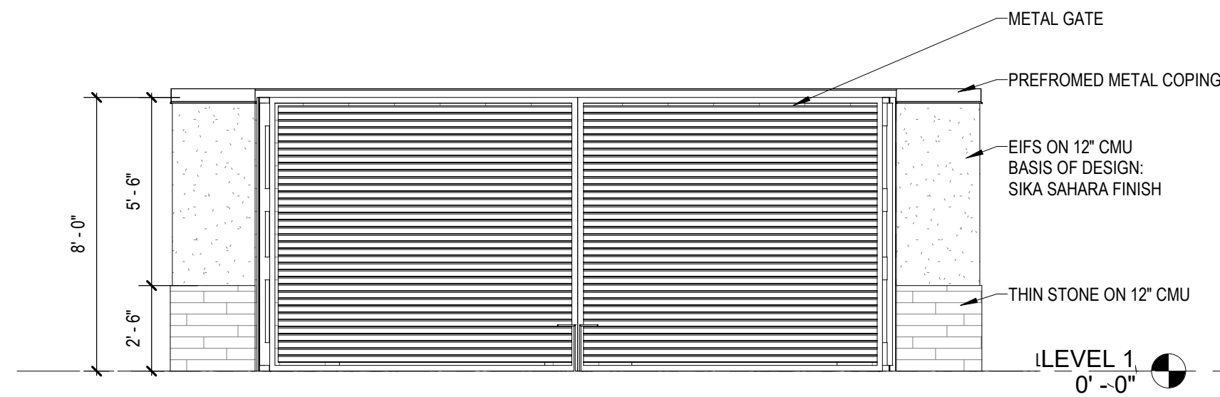
01 ELEVATION - DUMPSTER ENCLOSURE SOUTH AS1.03 1/4" = 1'-0"
