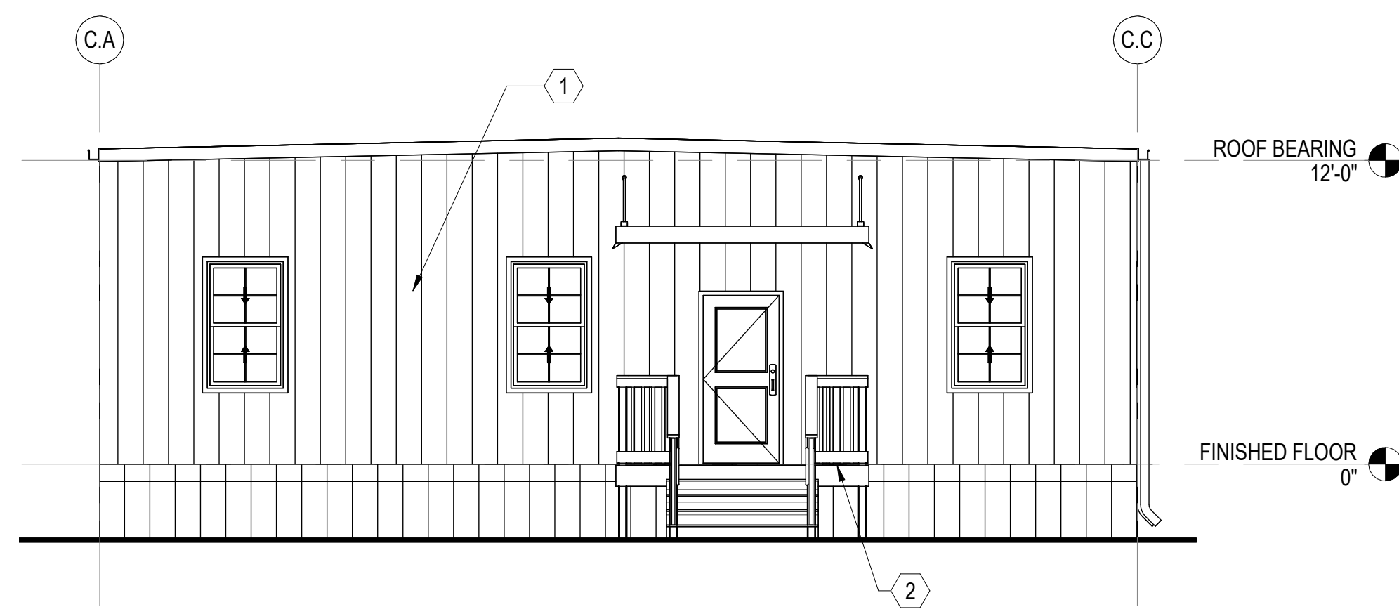
D MODULAR CLASSROOM WEST ELEVATION SCALE: 3/16" = 1'-0" (A-101)
