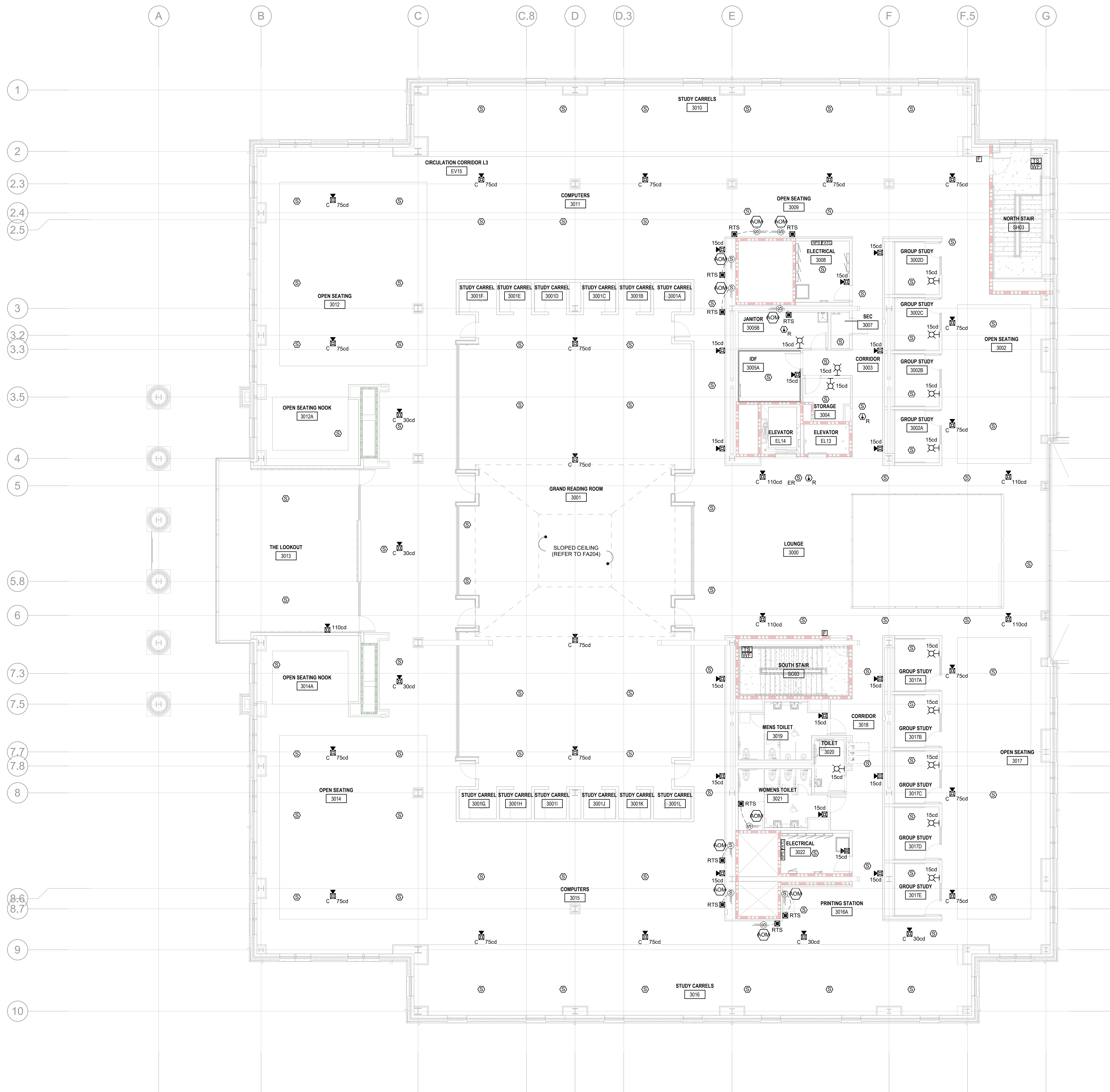
1 FIRE ALARM PLAN - LEVEL 3 - MAIN BUILDING SCALE: 1/8" = 1'-0"
