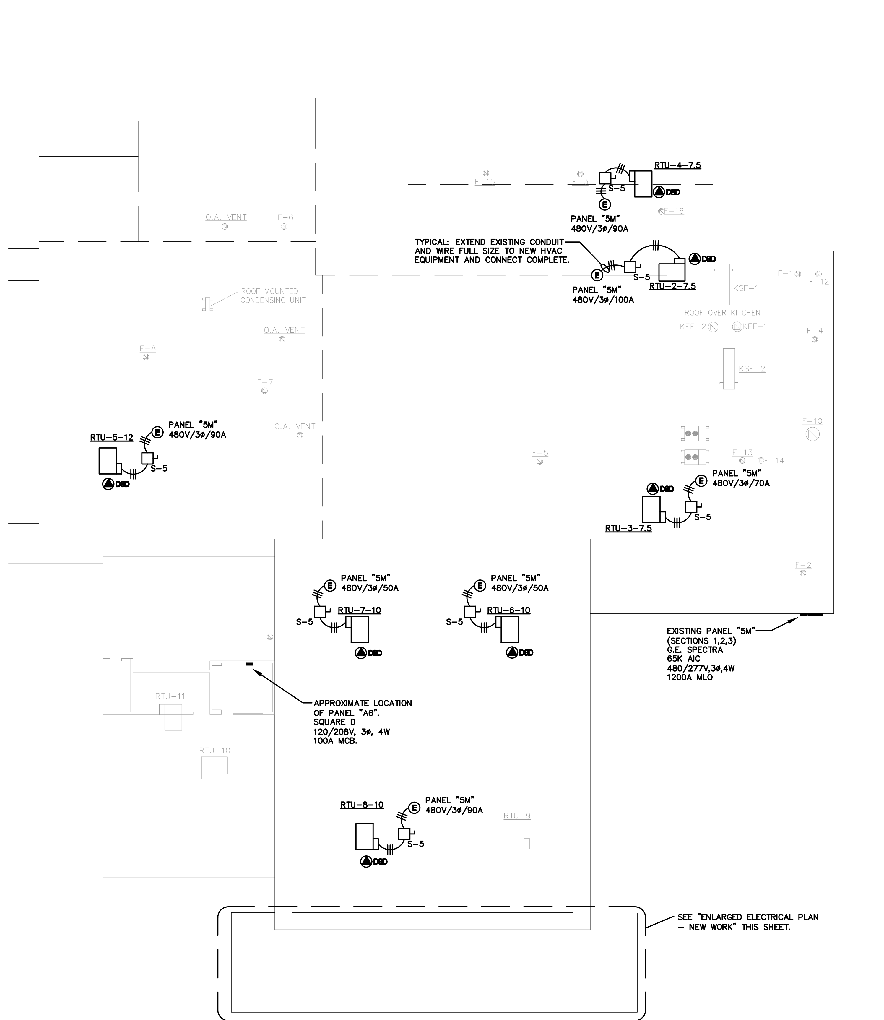
ELECTRICAL PLAN - NEW WORK - AREA "A" SCALE: 1/16" = 1'-0"
