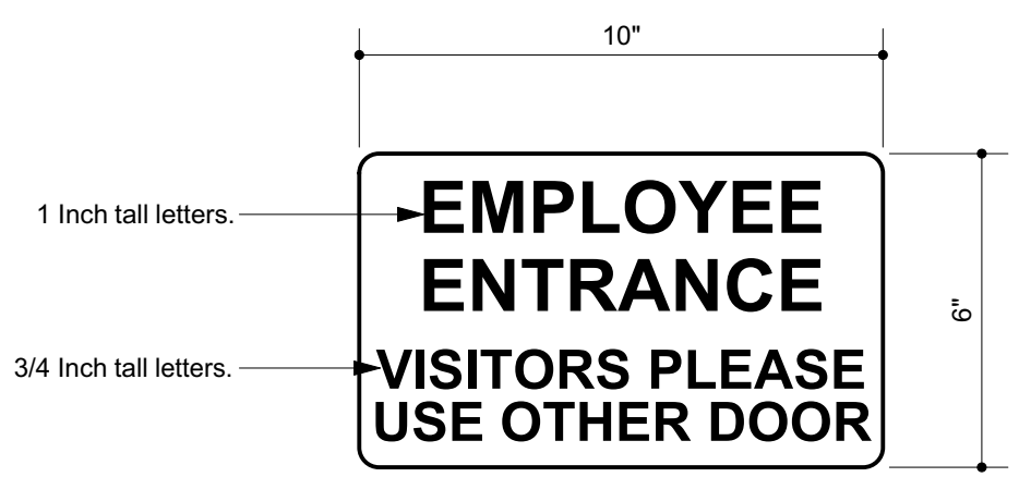
5 Wall-Mounted Sign Detail A6.0 Scale: 3" = 1'-0"
