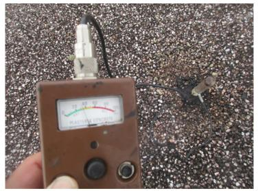
Photo 3 Meter confirmation of anomolie shown in photo #1.
