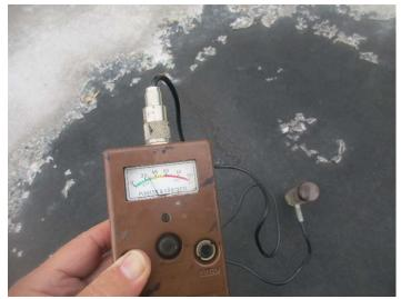
Photo 7. Meter showing minor moisture content from Photo 6.
