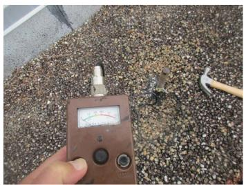
Photo 5. Meter did not confirm moisture in the roof @ Photo 4.
